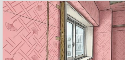
Renovated condominiums (phenolic foam boards)
