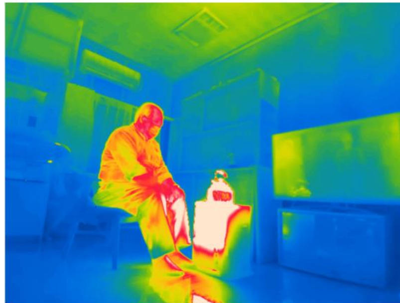
Before insulation and airtightness retrofit
